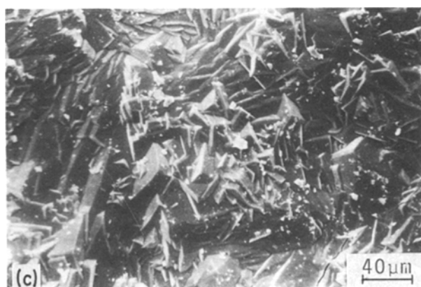
Figure 6 SEM photographs of the surfaces of \text{Si}_3\text{N}_4 layers. \text{Si}_2\text{Cl}_6 flow rate: 0.028 \text{ ml sec}^{-1} , \text{NH}_3 flow rate: 0.1 \text{ ml sec}^{-1} , \text{H}_2 flow rate: 1.0 \text{ ml sec}^{-1} , total gas pressure: 25 torr, deposition temperature: (a) 800^\circ \text{C} , (b) 1000^\circ \text{C} , (c) 1200^\circ \text{C} . (a) and (b) amorphous \text{Si}_3\text{N}_4 , (c) \alpha\text{-Si}_3\text{N}_4 .
